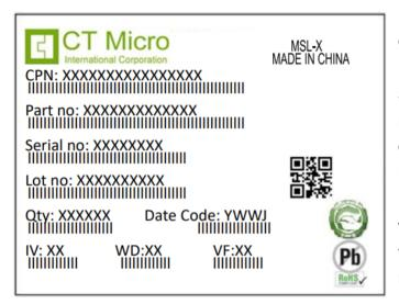
CPN : Customer Part Number Part no: CTM Production Number Serial no: Production Number Lot no: Lot number Q'ty: Packing Quantity Date Code: Manufacture Date IV : Bin Code of Luminous Intensity WD : Bin Code of Dominant Wavelength VF : Bin Code of Forward Voltage MADE IN CHINA: Production Place
